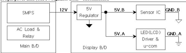
C. Split power Line (Separated 5V regulator used) – Strongly recommended
