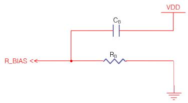
The  $R_BIAS$  is connected to the resistor to decide the oscillator and internal bias current. The sensing frequency, internal clock frequency and current consumption are therefore able to be adjusted with  $R_B$ . A voltage ripple on  $R_BIAS$  can make critical internal error, so  $C_B$  connected to the VDD (not GND) is recommended. (The typical value of  $C_B$  is 820pF and the maximum Value is 1nF.)
